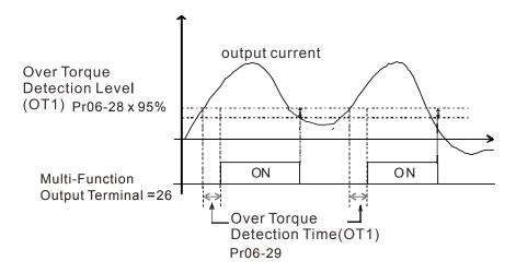
When Pr06-27 is set to 2 or 4, the ot1 fault will be displayed after Over Torque Detection. Then the motor drive stop running until it is manually reset.
