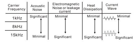
From the table, we see that the PWM carrier frequency has a significant influence on the electromagnetic noise, AC motor drive heat dissipation, and motor acoustic noise. If noises from ambient environment is greater than motor noise, lower PWM carrier frequency will help to lower the temperature of AC motor drive. When PWM carrier frequency is high, though the drive will operate more quietly, but wiring and interference may have problem.
